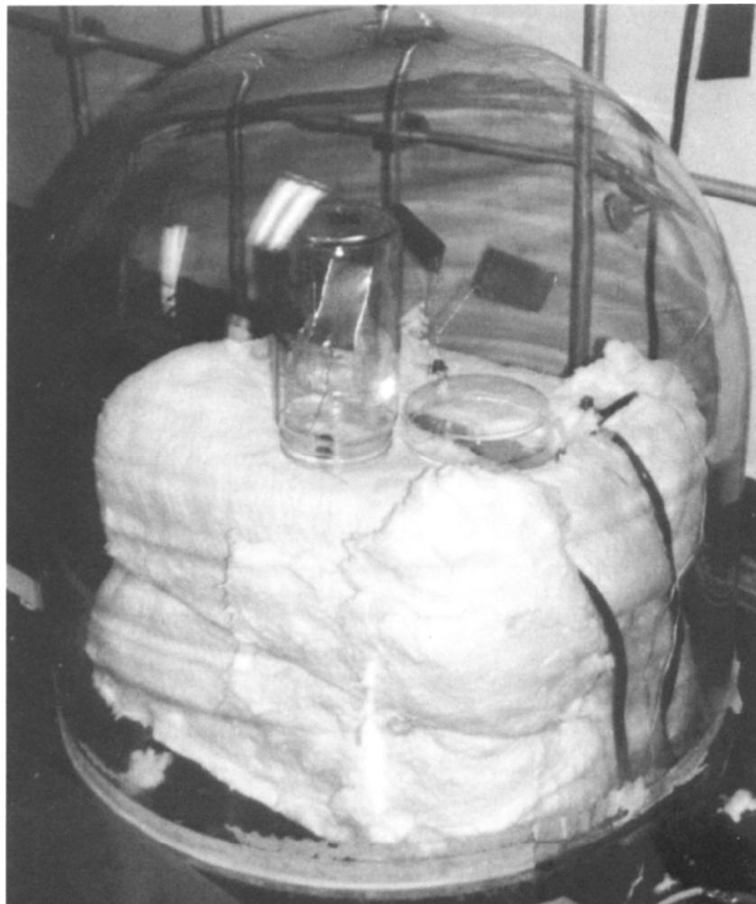
Fig. 1. Photograph of valve-regulated lead/acid battery, with thermal insulation, inside bell jar.
